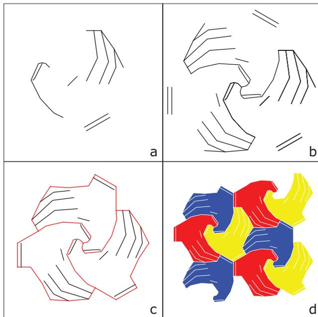
Figure 10: Workflow of tessellation. (design by Wouter Widdershoven)
