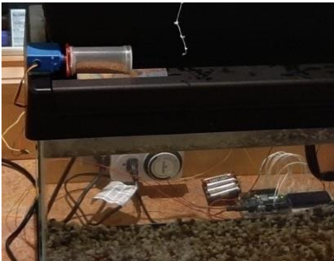
Figure 5. The second prototype for the automated fish feeder. (Source: Author)
